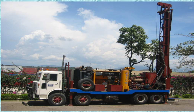
Drilling rigs like this drill deep small diameter boreholes. A pump is required to bring water to the surface. This method is expensive and inaccessible to most locations.
