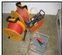
Some components of electrical resistivity surveying equipment.
